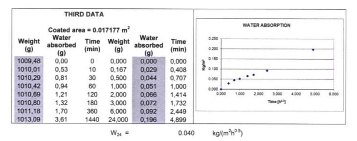
Coefficient of water absorption –  $w_{24} = 0.044 \pm 0.004 \text{ kg/(m}^2 \text{h}^{0.5})$
