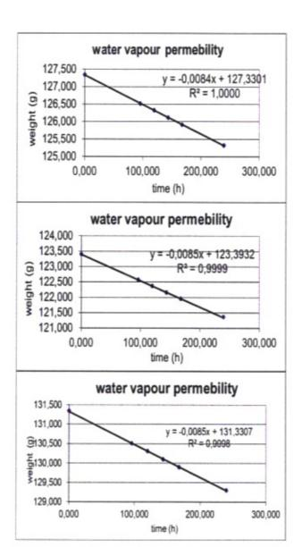
Starting from the resistance of the substrate (Sd = 0.0563 m) for the product in examination, the following average value of resistance to the transport is obtained:
